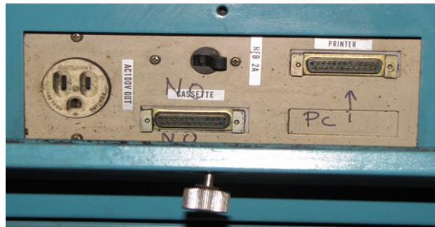
Figure 9: Mazatrol will probably have two DB25 female connectors, the one labeled Cassette must be used to save and load Mazatrol conversational programs. Sometimes the port is label with a picture of a cassette tape. The other DB25 is used only for EIA G code programs.
