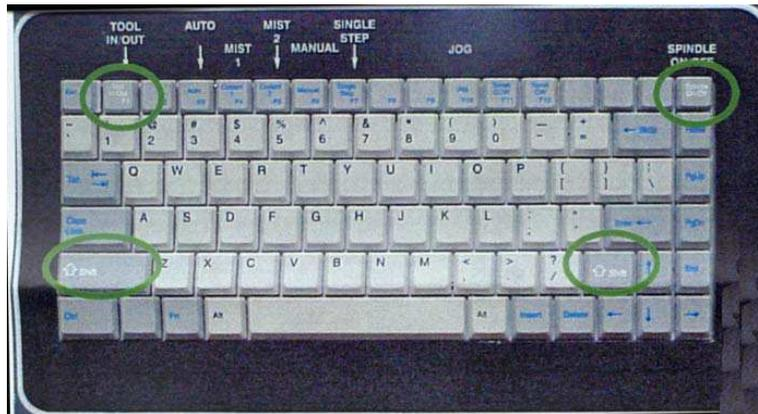
**Learn Mode** The Learn mode on the Fadal control has always been available, but when used on the TRM this feature can be very handy. As the machine is jogged to positions, the program can be built automatically. See the full description of this feature in the appropriate section of the Fadal User Manual.
