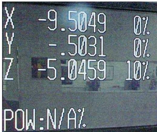
Figure 22-1 Full position display during manual mode (Jog)
